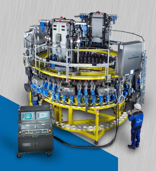
Multiple Stud Tensioner for Steam Generators PWR - Different Types & Sizes
