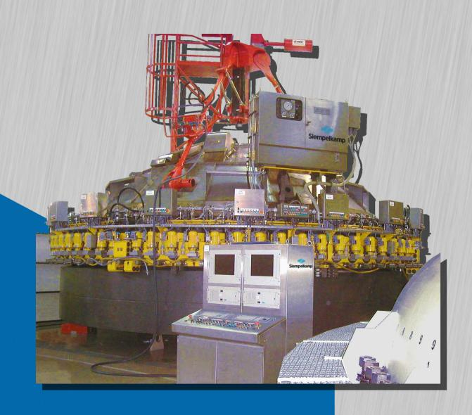
Multiple Stud Tensioning Machine for Boiling Water Reactors
